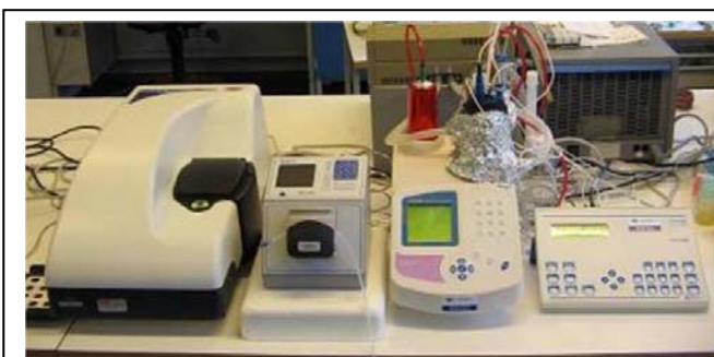
Figure 5 - Set-up for stirred batch reactor analysis of the physical and hydrochemical reactivity of ENPs under controlled atmosphere, pH, and temperature conditions. The system is based on a titrator for controlling the pH and on-line monitoring of average particle size by flow-cell DLS and changes in redox potential by redox electrodes connected to a multimeter. Stable physiological test temperature is enabled by using flow-cells connected to a temperature-controlled water-bath.
