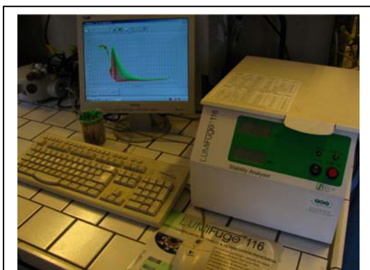
Figure 4 - The analytical photo-centrifuge at UniVE allows to give, in combination with DLS measurements, quantitative information on the stability of ENPs toward agglomeration and precipitation in various aqueous media and conditions.
